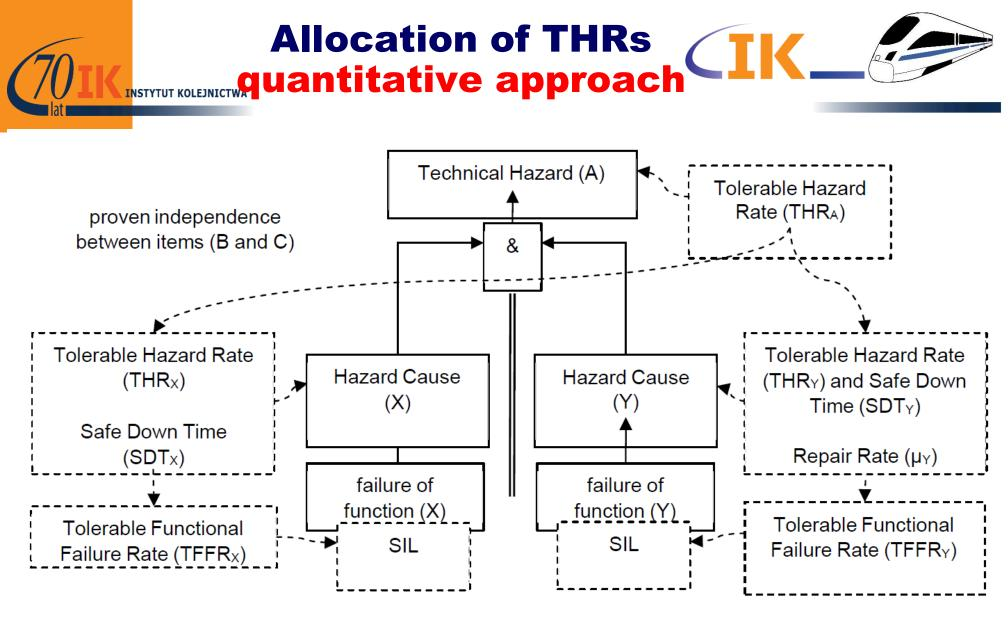
Allocation of the safety and reliability requirements as THR pointing Safety Integrity Levels (SIL) to functions and components [source: EN 50126-2]
